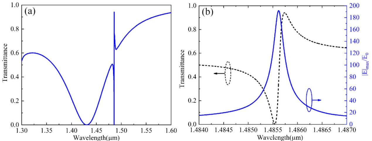
**Figure 3:** (a) Transmission spectrum through the slotted AlGaAs disk array with a linearly polarized plane wave excitation; (b) Zoom in showing the sharp resonance in (a), black dashed line. Also plotted in blue is the maximum of the local electric field amplitude in the AlGaAs domain as a function of wavelength.
