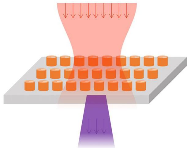
**Figure 1:** Schematic illustration of the second-harmonic generations (SHG) enhanced by the quasi-bound state in the continuum (QBIC) mode supported by slotted AlGaAs disk array. The red beam represents the incident wave at QBIC resonance while the outgoing purple beam is the generated second harmonic (SH) signal.
