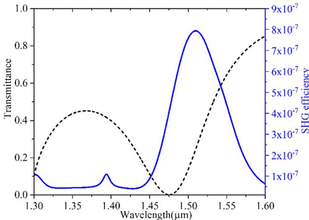
**Figure 5:** Transmission spectrum (dashed black line) and the second-harmonic generations (SHG) efficiency (blue line) from the magnetic dipole (MD) resonance supported by the AlGaAs disk array with no slot. Dimensions are similar to the slotted disk array.
