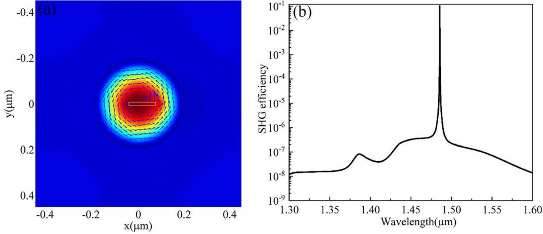
**Figure 4:** (a) Distribution of the magnetic field amplitude. Superimposed (blue arrows) is the vectorial orientation of the electric field inside the slotted disk at the wavelength of  $1.4855 \mu\text{m}$ ; (b) Calculated second-harmonic generations (SHGs) efficiency in the slotted AlGaAs disk array.
