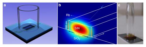
**Figure 1 | Atomic cladding waveguide illustration and photograph. (a)** Illustration of the ACWG. **(b)** Cross section of the SiN waveguide in the interaction area with the simulated fundamental TE mode superimposed. A Rb atom is illustrated as reflecting the surface, leaving the surface at a quenched state. **(c)** Photograph of the device showing the bonding of the vapour cell to the chip.
