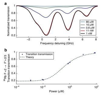
**Figure 3 | Nonlinear interaction in an atomic cladding waveguide.** (a) Normalized transmission of the ACWG with different incident power levels in the waveguide, attenuated using ND filters (b) Minimal transmission of the  $F = 2 \rightarrow F' = 2/3$  <sup>85</sup>Rb transition as a function of the optical power within the ACWG.
