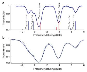
**Figure 2 | Atomic cladding waveguide spectroscopy.** (a) Natural Rb Doppler broadened spectrum, as measured through the cell attached to the silicon chip. (b) Normalized measured spectrum (blue solid line) and calculated spectrum (green dashed line). Calculations were performed based on the actual dimensions of the ACWG and the density of the vapour.
