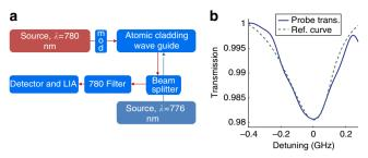
**Figure 5 | Two-photon absorption in an atomic cladding waveguide.** (a) Optical setup for measuring two-photon absorption in an atomic cladding waveguide. Mod, amplitude modulator; LIA, lock in amplifier (b) Measured transmission spectrum of the 780-nm source while being scanned by the 776-nm source (blue line), and the corresponding theoretical reference curve (green dashed line).
