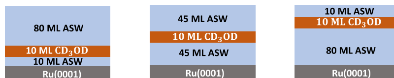
Figure 6. Schematic of position of 10 ML \text{CD}_3\text{OD} within ASW with a total film thickness of 100 ML.
